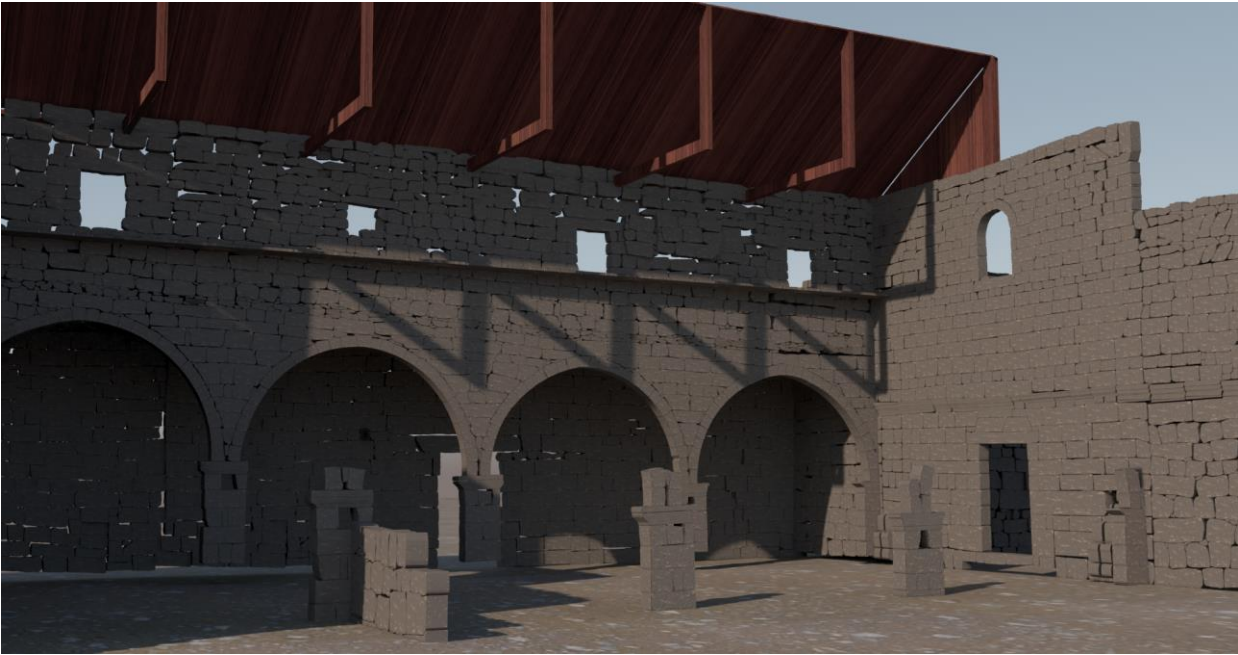
Figure 69: 3D section from northeast showing the roof, corbeling, arches inside the church, clerestory, and doors of the West church. Source: Author
